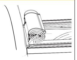
Roll up the cover. Do not disengage the hook and loop fasteners before rolling the cover. Always secure the cover at the front with both retainer straps.
