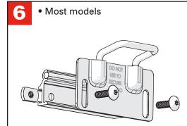
The brackets are assemblies comprised of the striker bracket (C), T-27 Torx screws (B), a backing plate (E) and a weld nut (D).
