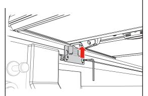
Align the striker brackets (C) so that the bracket loop aligns with and firmly latches into the cover latch assembly *(see step 8 for latch assembly adjustment)*. Attach to both driver and passenger sides. Using the provided T-27 Torx wrench, tighten the screws firmly while continuing to align the latches in later steps.
