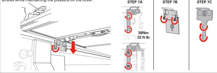
9 The tethers come installed on the bed cover hinge with a clamp at the other end. Install the clamp end by sliding the clamp onto the truck rail. Make sure the clamp is positioned as far up onto the rail as possible. Firmly hand tighten the knobs. Install the tethers on both sides of the cover.
