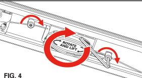
To make the final adjustment, loosen the striker bracket bolts or screws. Then move the bracket (C, F, H, or P) down by firmly pushing the cover (A) to the truck rail and tailgate. Make sure that both sides match, then retighten all the screws while maintaining the pressure on the cover.
