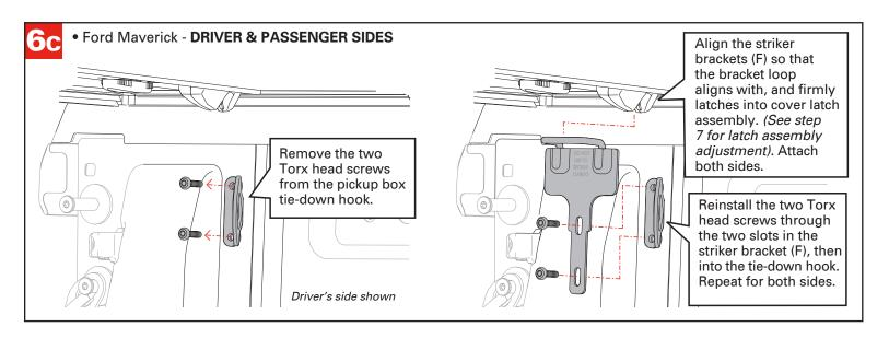
Adjustments and tightening of the latch assemblies are required.
