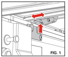
The bed cover latch assemblies and rotary knob come from the factory only partially tightened to allow installation adjustments. Both latches and rotary knob will require adjustment and final tightening. **Only use the hand tools provided, do not use power tools**.
