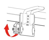
With the truck bed cover (A) closed, attach the striker brackets (C) to the metal truck bed rail.
