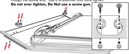
At the front/cab, fold the cab panel back and insert 2 mounting bolts through the keyed slots, on each side. When closed, the two bolts need to be aligned with the slotted bracket of the cover rails.
