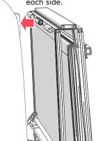
Position outer bumpers no closer than the one inch, or 25.4mm, from the outside edge of the panel as shown.
