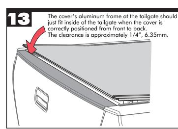
The rear edge of the cover and tailgate seal should rest on top of the tailgate. The cover must also be parallel with the tailgate
