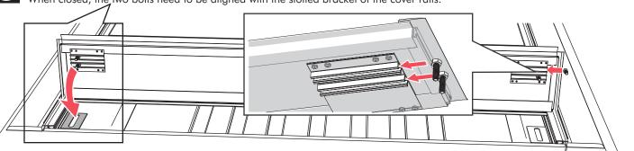
Install mounting hardware underneath the slotted bracket on the rail. Start with the rubber washer, then the large flat washer, then the nylon lock nut. Install two on either side.
