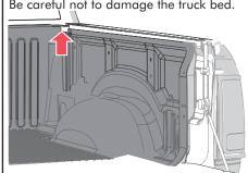
Make sure the rail is positioned square with the truck bed rail and firmly pressed to the bulkhead. Start with the middle clamp, placed in the center of the rail. Tighten the bolt enough to hold the clamp in place.
