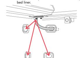
Install a cab bumper along the edge of the cover where it meets the truck cab taillight when in the propped up position. Other installations can benefit from the additional bumpers on each side.
