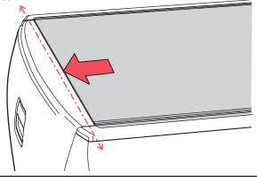
With the cover fully closed, check that the cover panel latches on both sides make proper contact with the side rails. Adjust the cover left to right so that both latches
