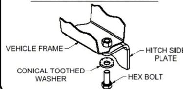
**PERIODICALLY CHECK THIS RECEIVER HITCH TO ENSURE THAT ALL FASTENERS ARE TIGHT AND THAT ALL STRUCTURAL COMPONENTS ARE SOUND.**
