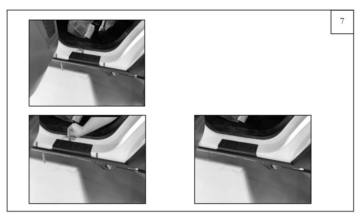
Set part in place on vehicle, sliding Trail Armor **underneath** the trim piece described in **Step 1**. Remove all red tapeliners. Apply FIRM pressure to mounting locations to affix to truck. Re-install screw removed in **Step 1**.
