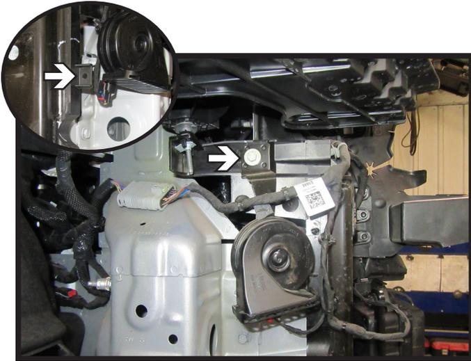
14. Unclip horn from the bracket (inset). Then using a 10MM socket, remove the one (1) bolt. Place the horn out of the way during baseplate installation, it will be reinstalled later. Do this on both sides of the vehicle.
