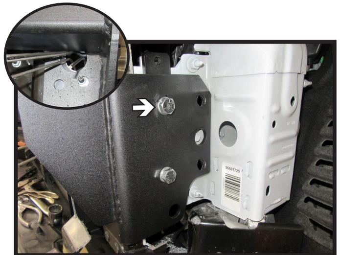
25. Insert spacer plate at top of baseplate between the frame and baseplate with the slotted end facing downward. Once spacer plate is in position insert 1/2" x 1-1/2" bolt with lock washer and whiz nut into top front hole (inset). Leave Loose Do this on both sides of the vehicle.
