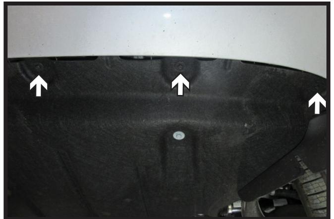
6. Using an 8MM socket, remove the five (5) bolts from the bottom of the fascia.
