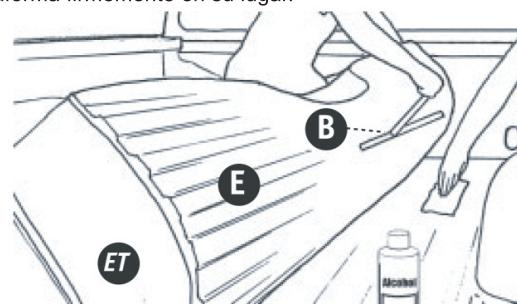
**8** Cut small slit for tie downs to protrude through liner.
