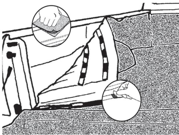
**10a** If your tuck bed is optioned with cargo lights, 110/230V outlet or assist handle, trim off section utilizing the trim lines located on the back side of the sidewalls.
