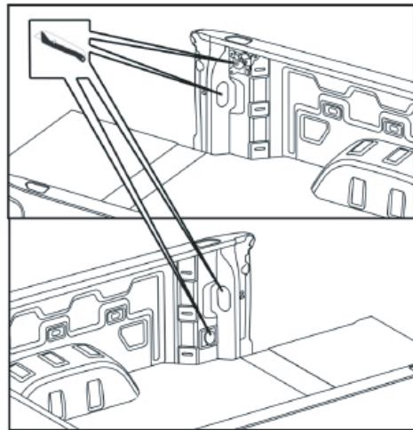
**11** Tailgate: Adhere tape just below the plastic cap. For Multipro tailgate, cut top tape as necessary. Remove mid gate panel section using scribe lines on back of carpet and install additional Hook fasteners at locations provided. (See 5a)
