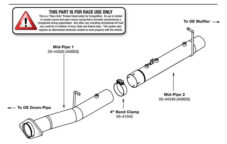
**Step 1:** (Read Instructions prior to installation) Disconnect sensors at the connections. Take caution as not to damage any sensors. Remove the CAT/DPF section of your trucks exhaust working your way forward. Take caution not to damage the factory isolation mounts as they will be reused. **It is recommended to not fully tighten the clamps until the entire system has been installed.**
