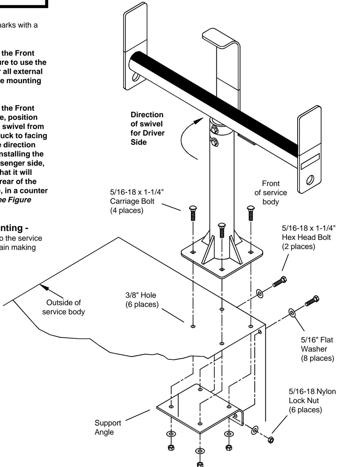
Figure 9. Front Stand Installation (shown on driver side)
