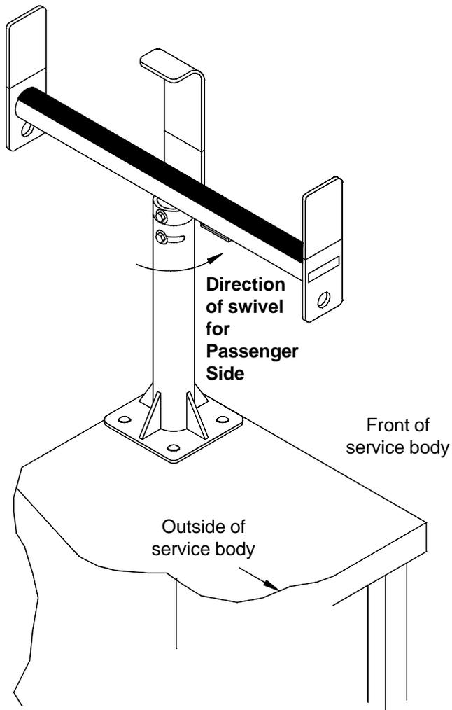
**Figure 10. Front Stand Installed (shown on passenger side)**
