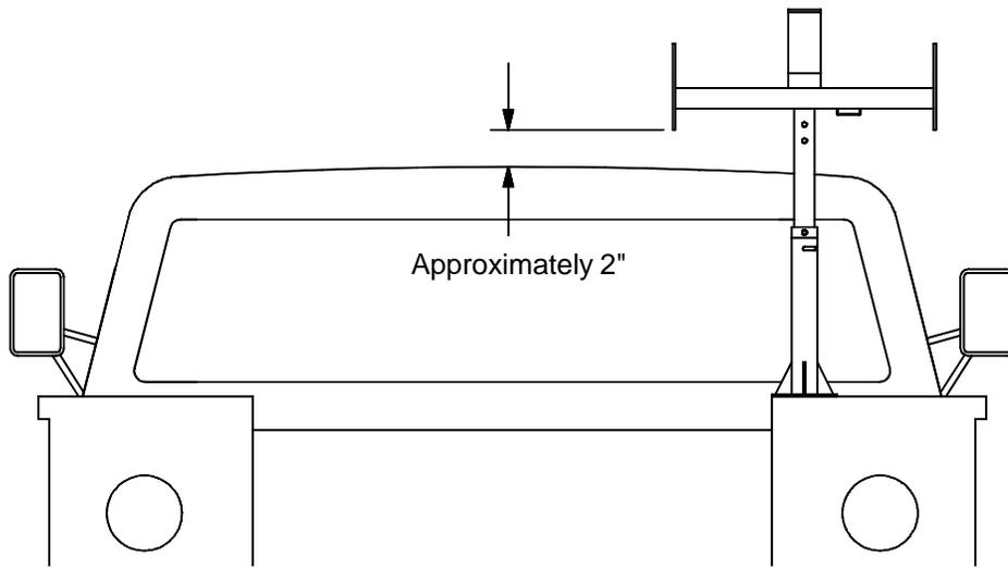
**Figure 4. Roof clearance**
