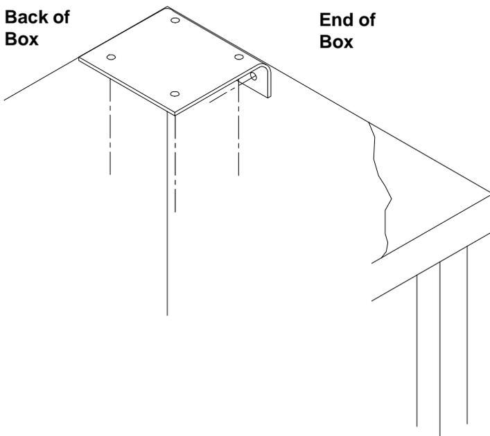
**Figure 7. Support Angle Placement (top & end panel)**
