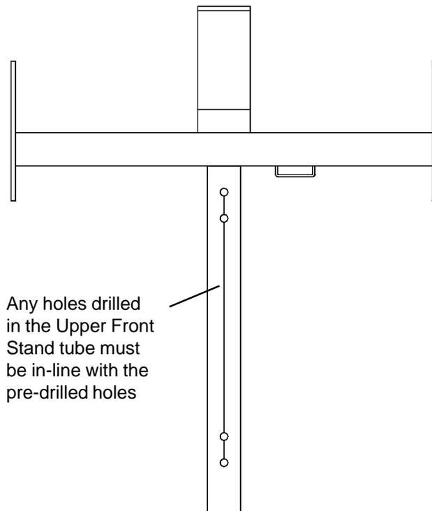
**Figure 3. Hole alignment**
