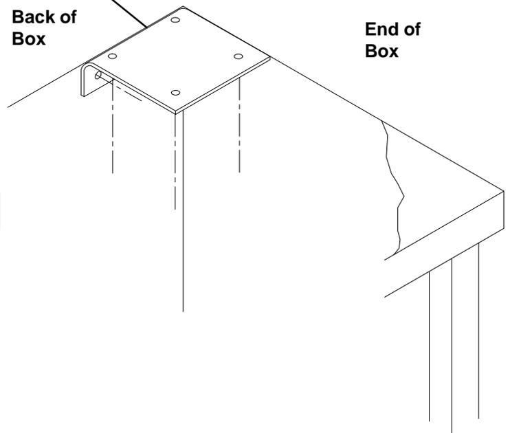
**Figure 8. Support Angle Placement (top & back panel)**
