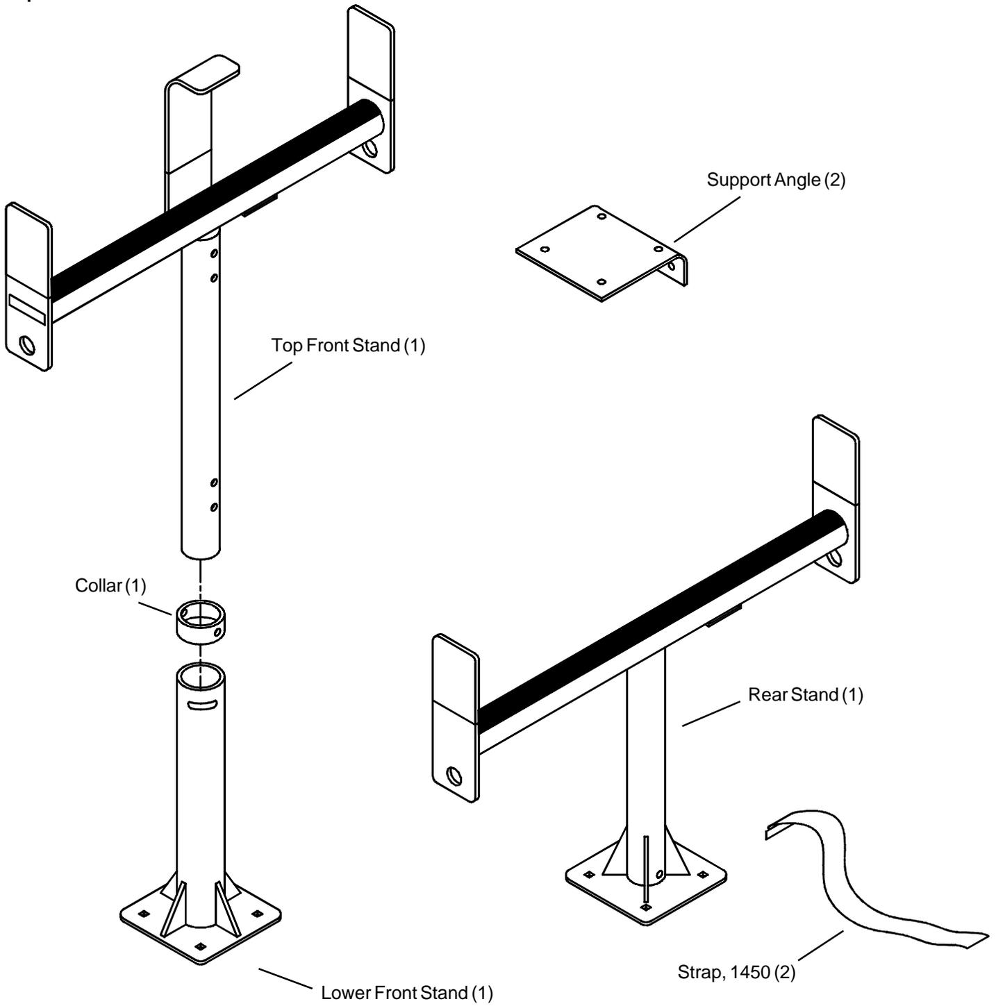
**Figure 1. Parts Identification**
